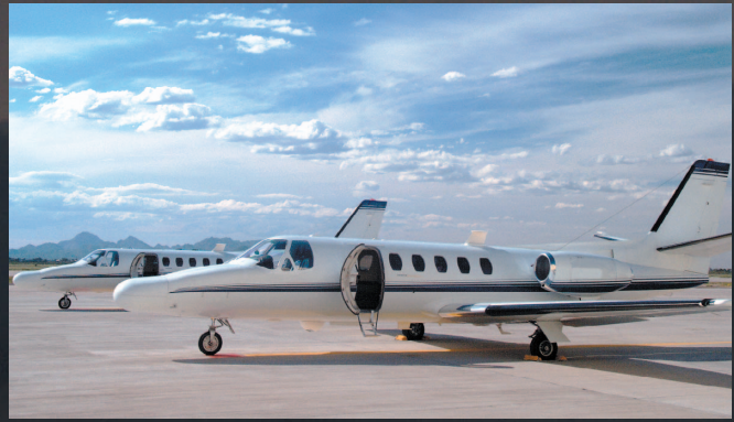
The 5 Cessna Citation IIs operated by CBP Tucson Air Branch have been heavily modified. They are fitted with millimeter wave radar, FLIR and low-light TV sensors to aid both in the hunt for UDAs and in assisting drug interdiction efforts.
