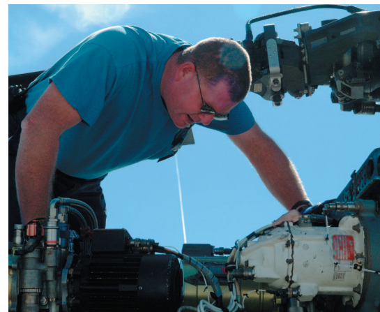
An L3 Vertex technician checks a small leak on a UH60 main rotor gearbox during a preflight inspection. When it was discovered that the leak emanated from an oil filter locking pin, the transmission was pulled and the pin repaired.
