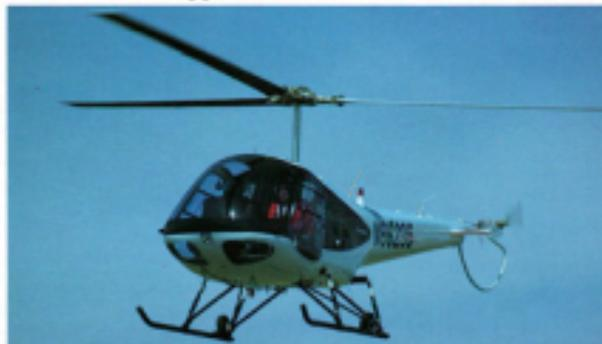
Enstrom's 280FX, powered by a six-cylinder Lycoming HO-360-F1AD, offers potential customers an alternative to the costs of turbine-powered helicopters.
