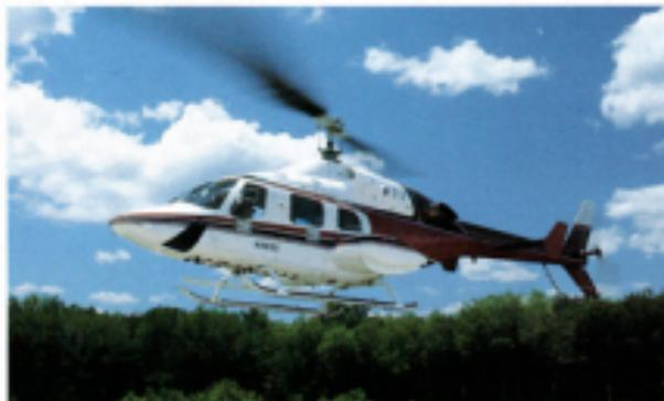
The twin-turbine Bell 222 is one of the few helicopters that customers may select with either a retractable landing gear or skids, as shown here on the 222UT.
