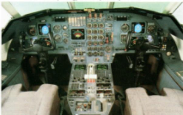
Like other new-generation heavy-iron business jets, the Dassault Falcon 900 includes the latest avionics and electronic instrumentation.
