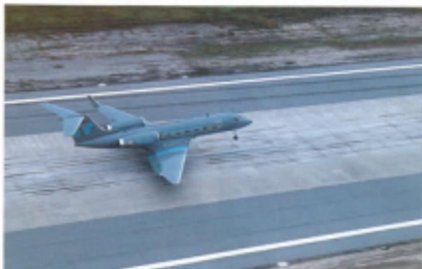
Spring marks the arrival of the long-awaited Gulfstream IV, which features a stretched fuselage, redesigned wing, new Rolls-Royce Tay powerplant and Sperry EFIS.
