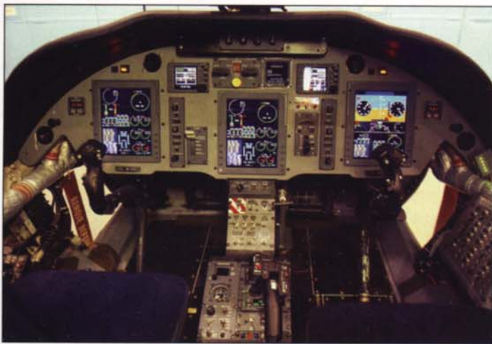
BA609 prototype cockpit uses Rockwell Collins Primus 21 display, nav-com and flight control systems, which will be standard on production aircraft. As the Primus 21 system is scalable, adding features such as EVS/SVS will be relatively simple.
