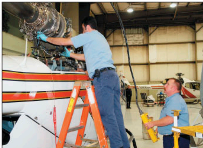
(L-R) Mechanics Chris Baboyan and Kevin Carver complete an engine change on one of the unit's EC120s. While the aircraft fulfills many of the missions it is tasked with, maintenance and performance issues have led SBCSD to purchase larger, more powerful AS350B3 AStars.
