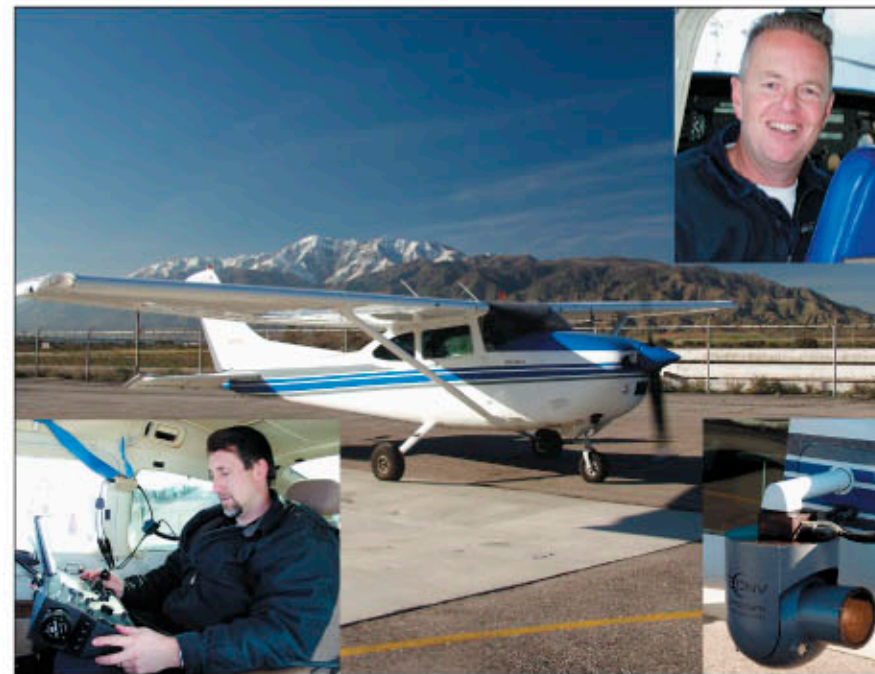
The SBCSD Cessna 182 at L69 (Rialto CA). According to Pilot Shawn Moore (inset R) and Observer Mike Brownie (inset L), the GyroCam DNV system is sharp enough to read a license plate from an altitude of 5000 ft AGL. Equipped with a laser illuminator for night IR sensing, the aircraft and its systems are used throughout the county and into neighboring Los Angeles.
