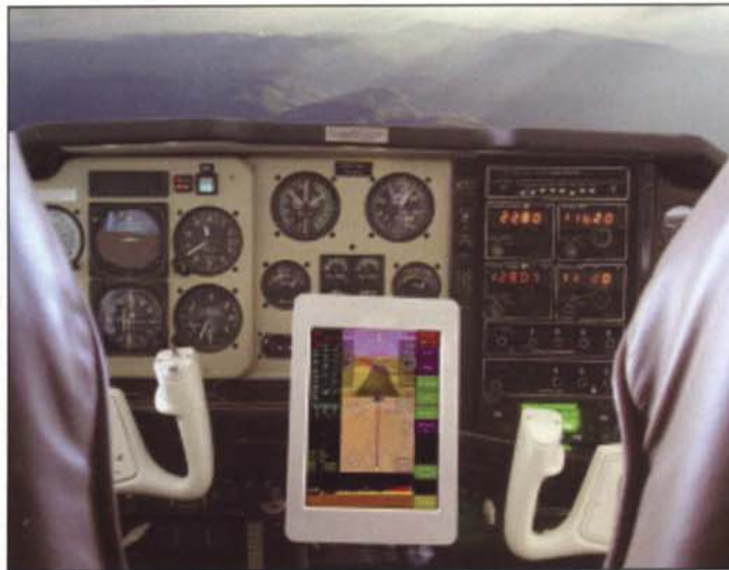
At present, certified synthetic vision systems are relatively expensive. NASA has tasked Operator Performance Laboratory (OPL) with researching optimal display characteristics of a low-cost SVS. OPL's Synthetic Flight Bag, shown here, is the result.
