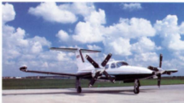
The evolution of the T-tail Cheyenne reached its zenith with the 400LS, Piper Aircraft Corporation's Garrett-powered 400-mph turboprop.
